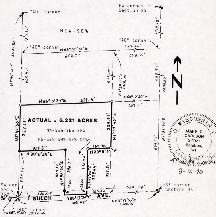
Bearings are referenced to east line of SE¼ of Section 35 and assumed to bear N1°34'40"E.
