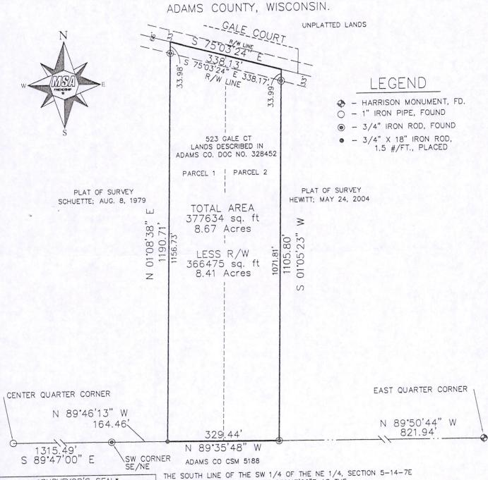
THE SOUTH LINE OF THE SW 1/4 OF THE NE 1/4, SECTION 5-14-7E WAS ASSIGNED A BEARING OF S89.47'00"E AS THE BASIS OF BEARINGS ON THIS MAP.
