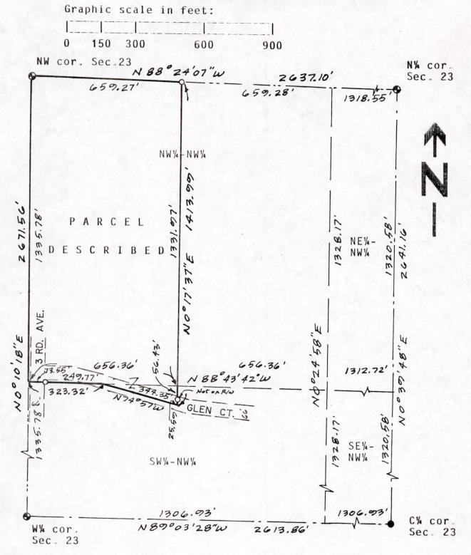
Bearings are referenced to the west line of the NW% of section 23 and assumed to bear N0°10'18"E.
