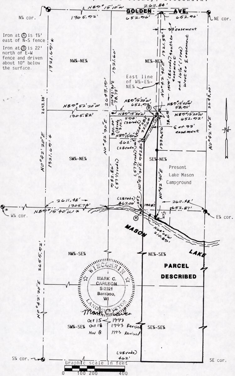
Bearings are referenced to the east line of the NE% of Section 26 and assumed to bear N0°42'40"E and rounded to nearest 10".
