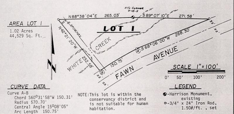
NOTE:North line  $NE\frac{1}{4}$  3-15-5 assigned  $S89^{0}07'10''E$  for bearings on this map.
