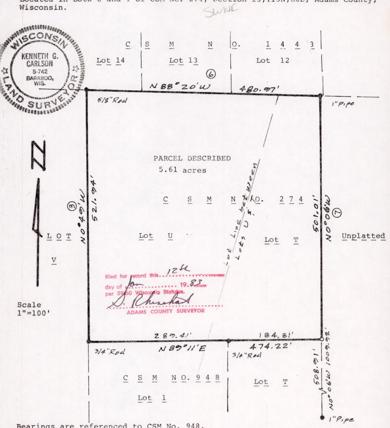
Bearings are referenced to CSM No. 948. •= Found iron as shown. O = Set 3/4"x24" round iron rod weighing 1.5 #/lineal Lines recorded as: 3 N0°01'54"E, 6 N88°40'34"W, 481.497', 7 N0°00'35"E, 1007.664'.
