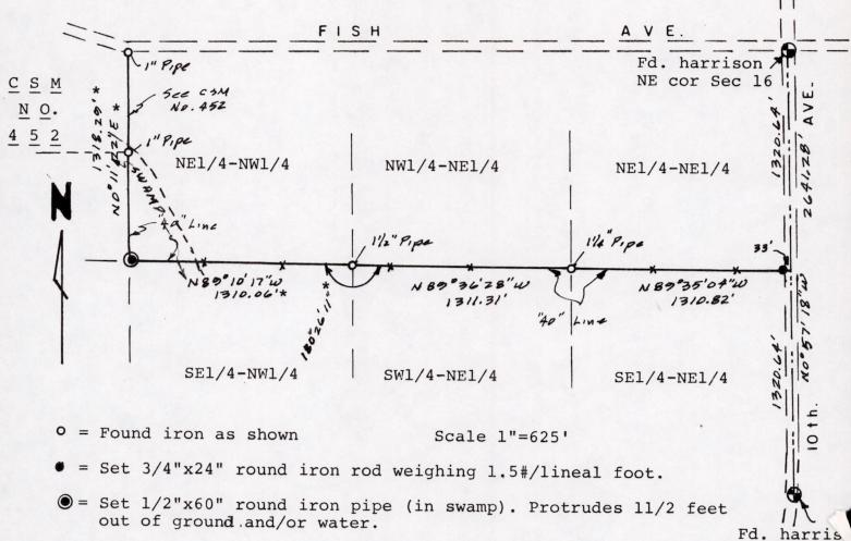
El/4 cor. x = Set 5 foot steel fence post on line and also next to irons Sec. 16 set and found.
