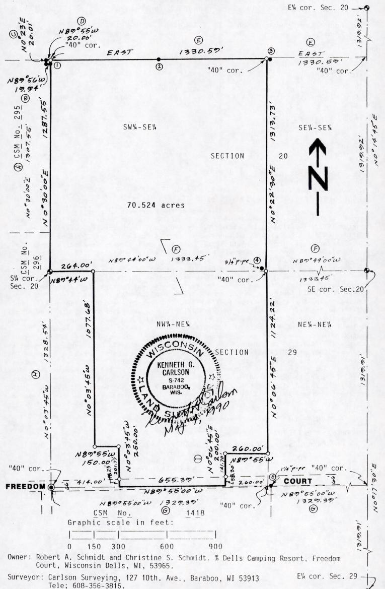
Bearings are referenced to the south line of the SE% of Section 20 and assumed to bear N89°44'00"W and rounded to nearest 15".
