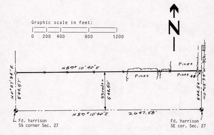
Bearings are referenced to the south line of the SE¼ of Section 27 and assumed to bear  $N89^{\circ}10'40"E$ , the same as Section Summary by L. Scott of 8/6/81. Other bearings shown are also taken from same Section Summary.
