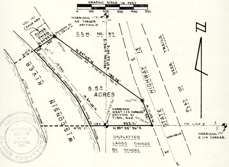
Bearings are referenced to the west line the NW 1/4 of Section 31 and assumed to bear N 0°23'05" E.
