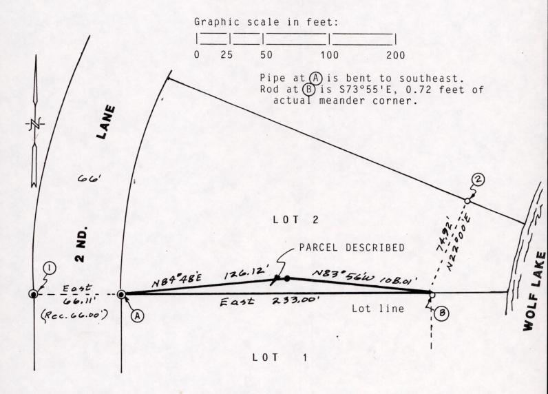
Bearings are referenced to the plat of Wolf Lake using the irons found at  $\bigcirc$  and  $\bigcirc$  which were used to determine boundaries of survey.
