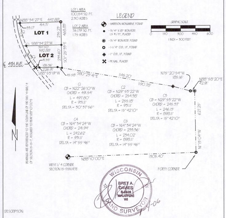
Commencina at the West 1/4 comer of said Section 15, thence N88°10'00''E, 1305,40 feet to the 1/16th comer and an Iron Pipe; thence N01°13'04''W, 627.25 feet along the 1/16th line; Thence N88° 58' 20" E, 42.91 feet; thence N75° 20' 54" W, 185.16 feet; thence N80° 23' 41" W, 1145.20 feet to the POINT OF BEGINNING:
