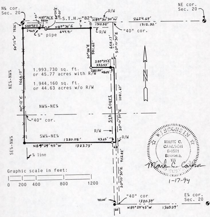
Bearings are referenced to north line of NE% of Section 20 and assumed to bear N89°30'30"W.
