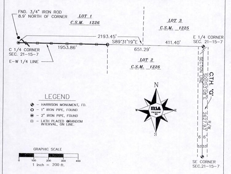
THE EAST—WEST QUARTER LINE OF SECTION 21-15-7 WAS ASSIGNED A BEARING OF N89'31'18"W AS THE BASIS OF BEARINGS ON THIS MAP.
