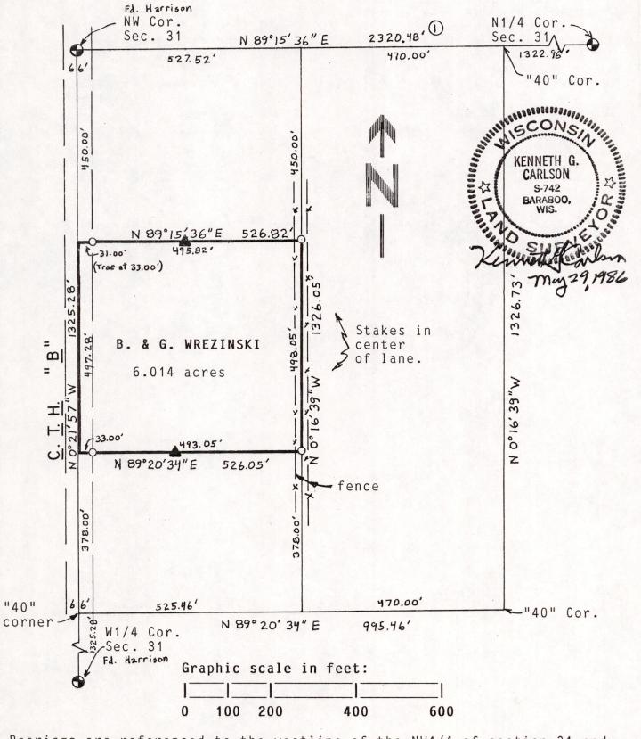
Bearings are referenced to the westline of the NW1/4 of section 31 and assumed to bear N0°21'57"W, the same bearing as section summary by F. Zietlow of 8-24-77. The same section summary was used to subdivide the section to get the dimensions shown on the map.
