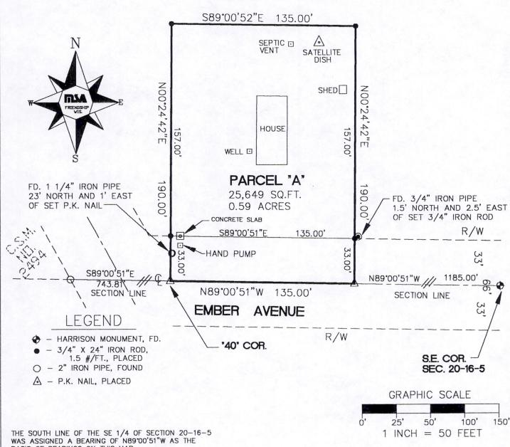
THE SOUTH LINE OF THE SE 1/4 OF SECTION 20-16-5 WAS ASSIGNED A BEARING OF N89 00 51 W AS THE BASIS OF BEARINGS ON THIS MAP.
