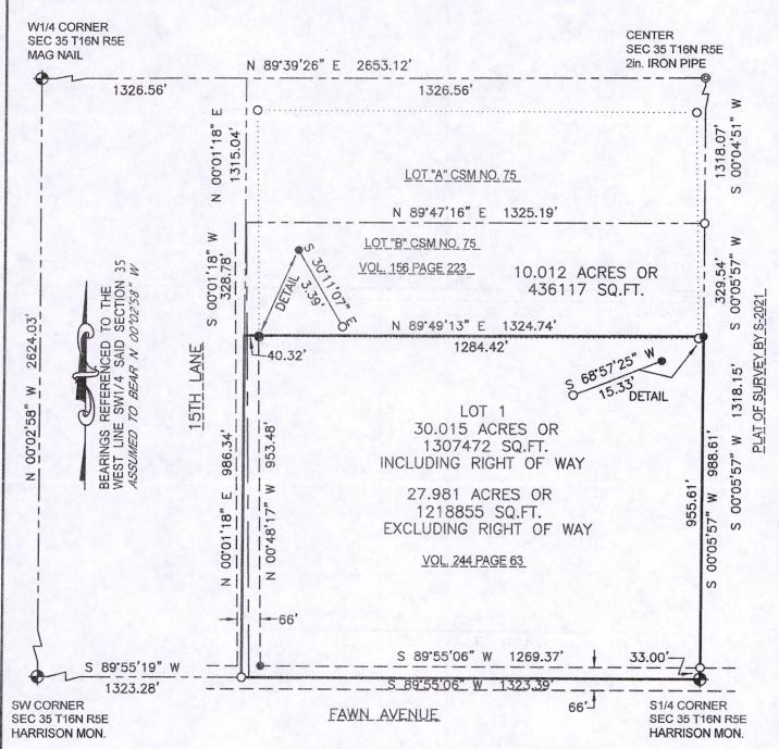
SURVEYORS NOTE: BECAUSE OF THE DISCREPANCIES IN CSM NO. 75 THE SE1/4 OF THE SW1/4 WAS STAKED USING VOL. 156 PAGE 223 AND VOL. 244 PAGE 63.
