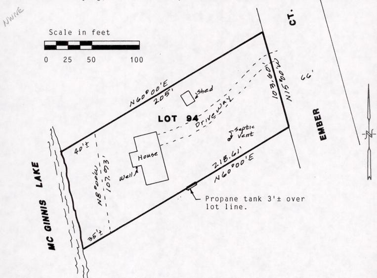
Bearings and distances shown are from the recorded plat and are not checked for accuracy.
