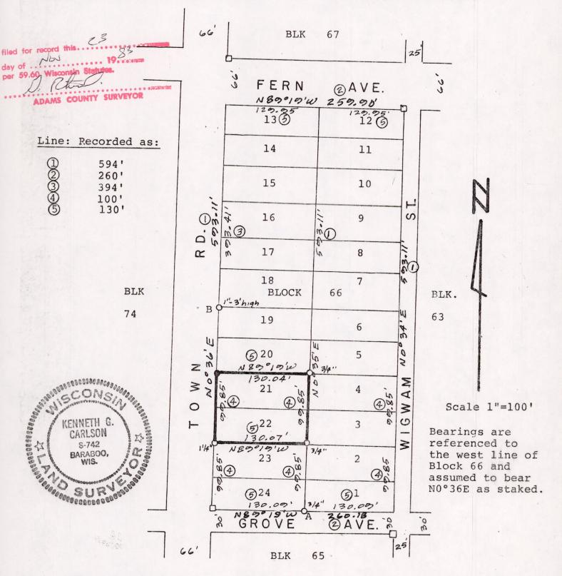
$\Box$ = Found 3/4" or 5/8" square iron bar from original survey.  $\circ$  = Found iron pipe as shown.  $\circ$  = Set 3/4"x24" round iron rod weighing 1.5#/lineal foot.
