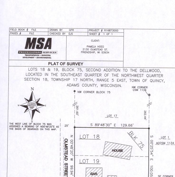
BLOCK 92 75 GRAPHIC SCALE SW CORNER BLOCK 75 LEGEND 60 30 40 1 INCH = 40 FEET 100 - 3/4" SQ. IRON ROD, FOUND \*SURVEYOR'S SEAL\* 1" IRON PIPE, FOUND NW CORNER BLOCK 76
