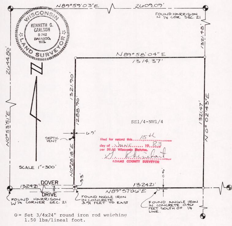
Bearings are referenced to the N-S 1/4 line of Section 21 and assumed to bear N0°02'43"E. Survey used the Section Summary by Kiedrowski Engineering dated 10/30/80 and tied into the SW, W1/4, and N1/4 corners of Section 21.
