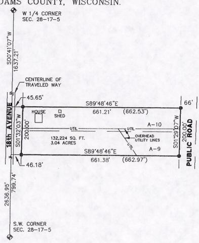
THE WEST LINE OF THE SW 1/4 OF SECTION 28-17-5 WAS ASSIGNED A BEARING OF S00'41'07"W AS THE BASIS OF BEARINGS ON THIS MAP.
