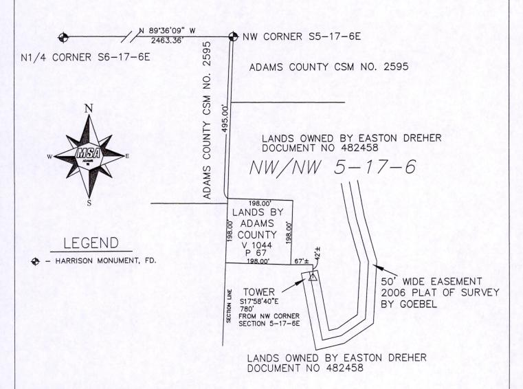
THE NORTH LINE OF THE NE 1/4 OF SECTION 6-17-6E WAS ASSIGNED A BEARING OF N89\*36'09"W AS THE BASIS OF BEARINGS ON THIS MAP.
