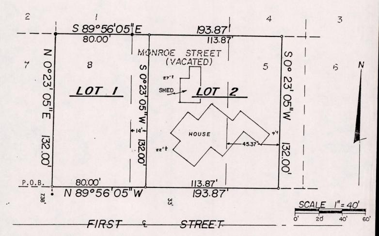
NOTE: The east line of Lot 8, Block 1 was assigned a bearing of S  $0^{\circ}23'05"W$ as the basis for the bearings on this map.
