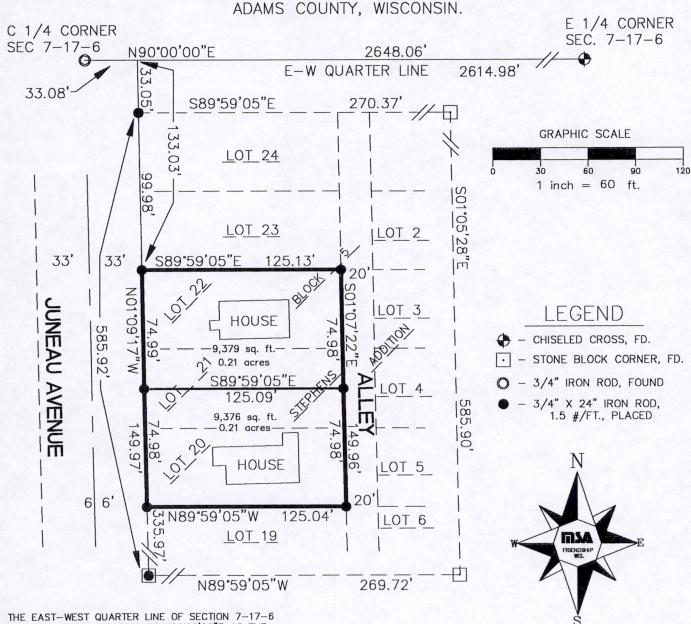
THE EAST-WEST QUARTER LINE OF SECTION 7-17-6 WAS ASSIGNED A BEARING OF N90 $^{\circ}00^{\circ}00^{\circ}E$  AS THE BASIS OF BEARINGS ON THIS MAP.
