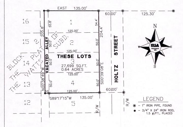
THE SOUTH RIGHT OF WAY LINE OF GROVE STREET SECTION 8-17-6 IS ASSUMED TO HAVE A BEARING OF EAST AS THE BASIS OF BEARINGS ON THIS MAP.
