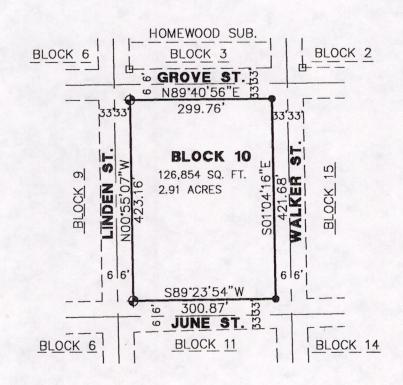
THE WEST LINE OF BLOCK 10 OF THE RAILWAY ADDITION TO FRIENDSHIP WAS ASSIGNED A BEARING OF NO0°55'07"W AS THE BASIS OF BEARINGS ON THIS MAP.
