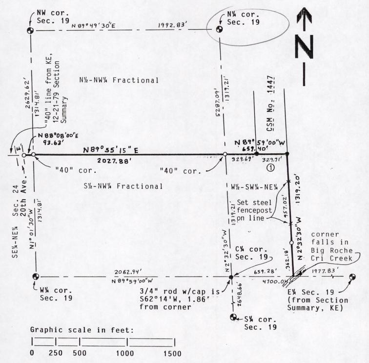
Bearings are referenced to west line of Fractional NW% and assumed to bear N0°01'30"W.
