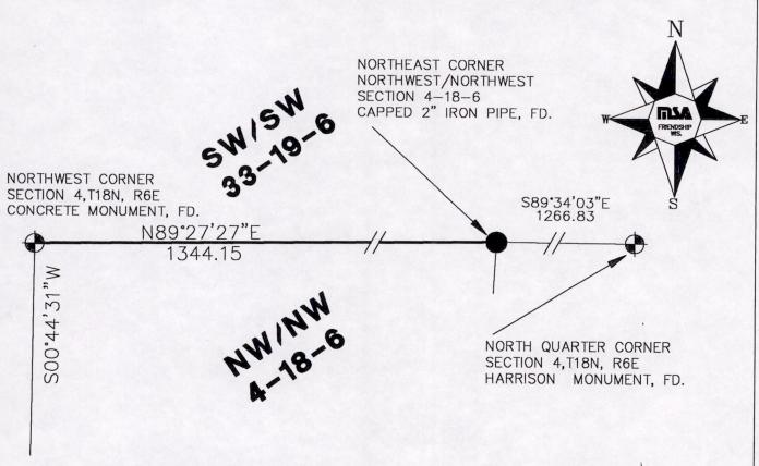
NOTE: 7/8 " O.D. IRON RODS OR 1" O.D. IRON PIPES, 5 FEET LONG, WERE DRIVEN AT RANDOM INTERVALS ALONG THE NORTH LINE OF THE NW/NW AND ABOUT 100 FEET SOUTH FROM THE NORTHWEST CORNER ON THE WEST LINE. THE IRONS WERE DRIVEN WITH ABOUT 2 FEET EXPOSED.
