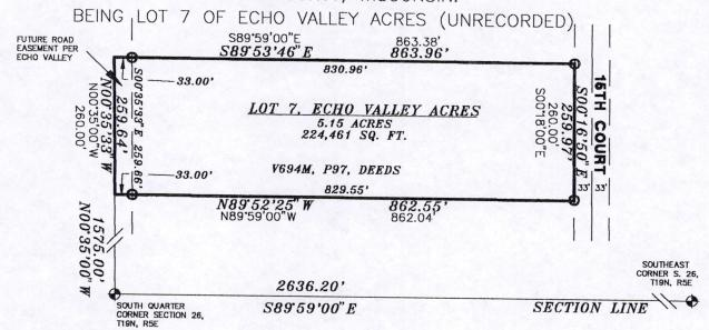
THE SOUTH LINE OF THE SE 1/4 OF SECTION 26-19-5 WAS ASSIGNED A BEARING OF S89'59'00"E AS THE BASIS OF BEARINGS ON THIS MAP.
