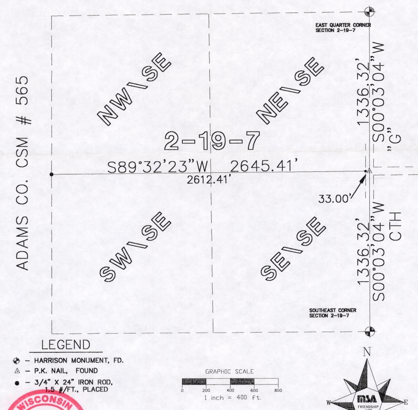
THE EAST LINE OF THE SE 1/4 OF SECTION 2-19-7 WAS ASSIGNED A BEARING OF S00.03'04"W AS THE BASIS OF BEARINGS ON THIS MAP.
