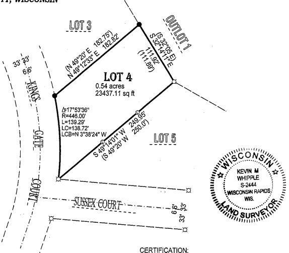
() RECORDED AS 3/4" IRON ROD FOUND X2" O.D. IRON PIPE FOUND (L) WOOD LATH BASIS OF BEARINGS: THE SOUTH LINE OF LOT 4 ASSIGNED A BEARING OF S 49°14'01" W FOR THIS MAP
