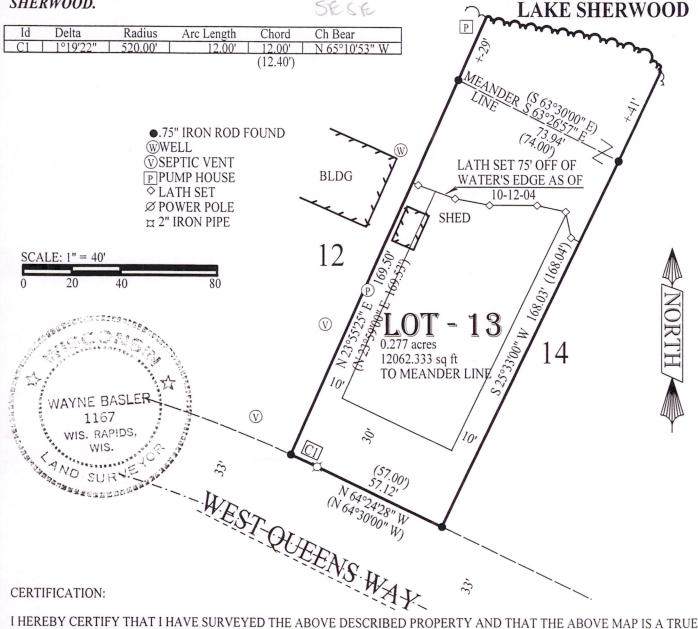
I HEREBY CERTIFY THAT I HAVE SURVEYED THE ABOVE DESCRIBED PROPERTY AND THAT THE ABOVE MAP IS A TRUE REPRESENTATION THEREOF AND SHOWS THE SIZE AND LOCATION OF PROPERTY, ITS EXTERIOR BOUNDARIES, THE LOCATION OF ALL VISIBLE STRUCTURES THEREON, BOUNDARY FENCES, APPARENT EASEMENTS, ROADWAYS AND VISIBLE ENCROACHMENTS, IF ANY. THIS SURVEY IS MADE FOR THE USE OF THE PRESENT OWNERS OF THE PROPERTY, AND THOSE WHO PURCHASE, MORTGAGE, OR GUARANTEE TITLE THERETO WITHIN ONE YEAR FROM THE DATE HEREOF.
