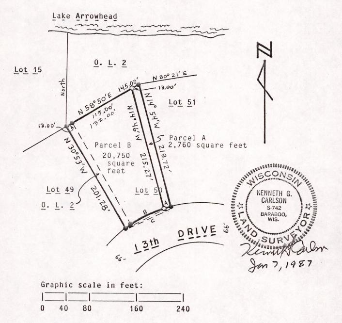
O = Set 3/4"x24" round iron rod weighing 1.5#/lineal foot. = Found 3/4" round iron rod.
