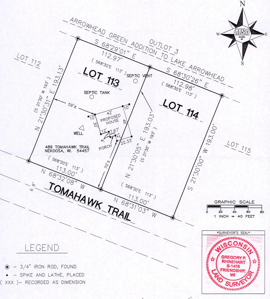
THE EASTERLY LINE OF LOT 114 WAS ASSIGNED A BEARING OF S21°30'00"E AS THE BASIS OF BEARINGS ON THIS MAP.
