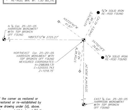
(e) Describe any material discrepancy between the location of the corner as restored or re—established and the location of that corner as previously restored or re—established by distance and direction. Show the discrepancy on the plan view drawing under (d), above. Show the distances between the corner as previously restored or re—established and (1) the corner as restored or re—established, and (2) to at least 2 of the 4 witness monuments shown on the drawing in (d), above.
