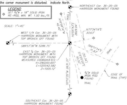
(e) Describe any material discrepancy between the location of the corner as restored or re—established and the location of that corner as previously restored or re—established by distance and direction. Show the discrepancy on the plan view drawing under (d), above. Show the distances between the corner as previously restored or re—established and (1) the corner as restored or re—established, and (2) to at least 2 of the 4 witness monuments shown on the drawing in (d), above.
